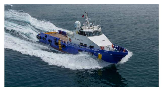
Two 33.5-meter fast aluminum crew boats have been delivered to Fujairah National Group. The vessels are an optimized version of the successful in-house design built to help with fast transfer of offshore personnel, deck cargo and liquid payload.
