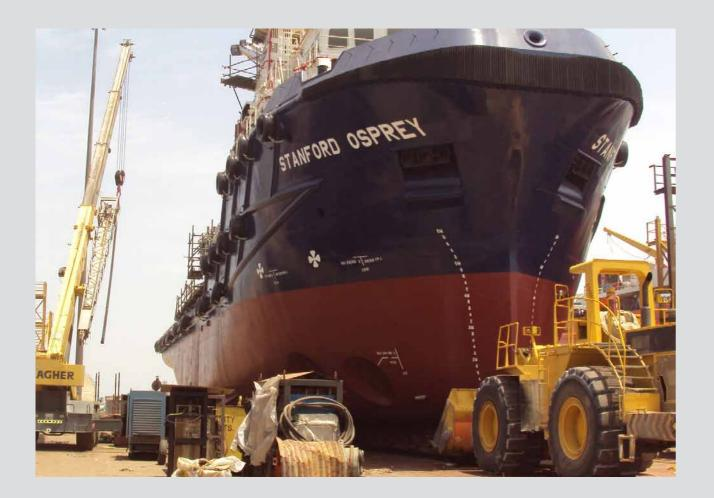
Grandweld has successfully upgraded MV Stanford Osprey during April and May this year. New power and redundancy requirements as per ABS DPS2 notation have resulted in moving from DP1 to DP2 classification.
