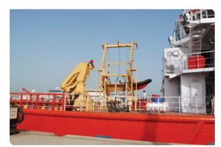
Davit and crane installed on top of new module deck
