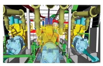
3D modeling of machinery, piping & electrical for optimized layouts and maintainability.
