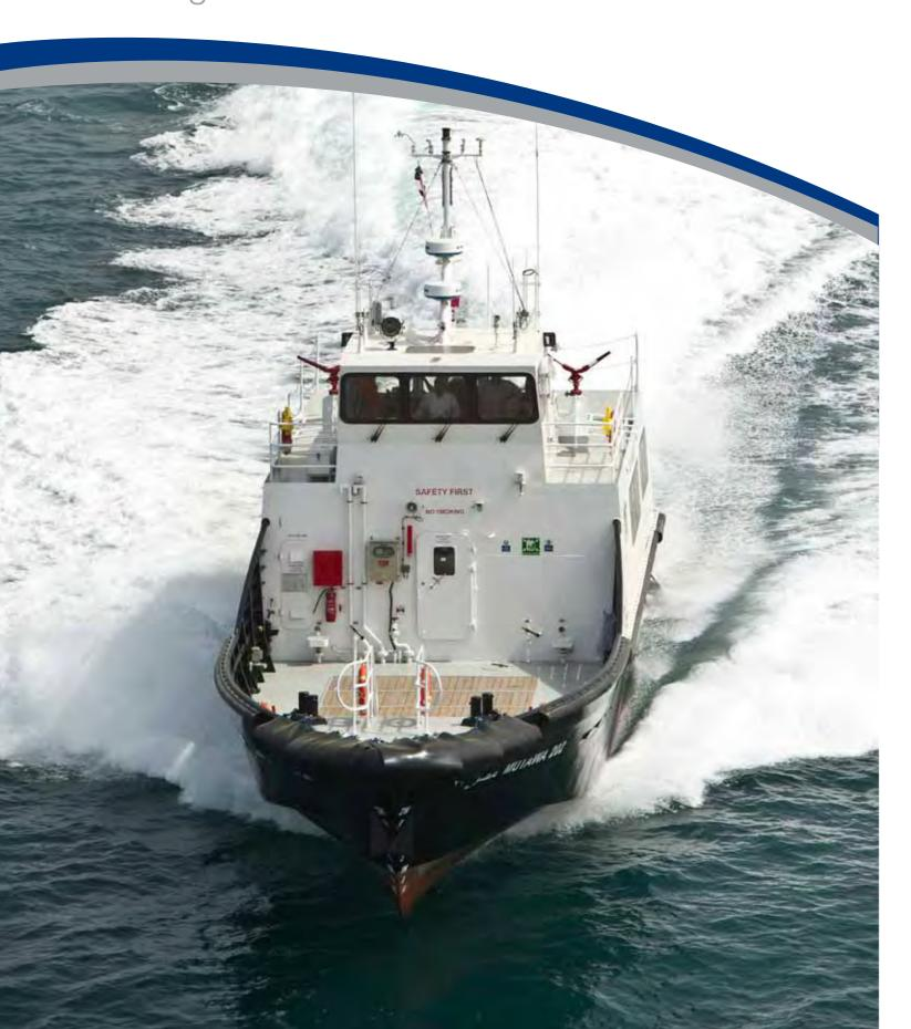
Grandweld Shipyards delivers the first forward landing crew boat design in the region. The 24M vessel features a customized forward bow fender, designed for steady and secure landing into a dedicated offshore landing structure. Upon swift landing, the offshore personnel can directly disembark to the offshore platform. This feature allows for safe, stable and quick embarkation of passengers to the offshore site.
