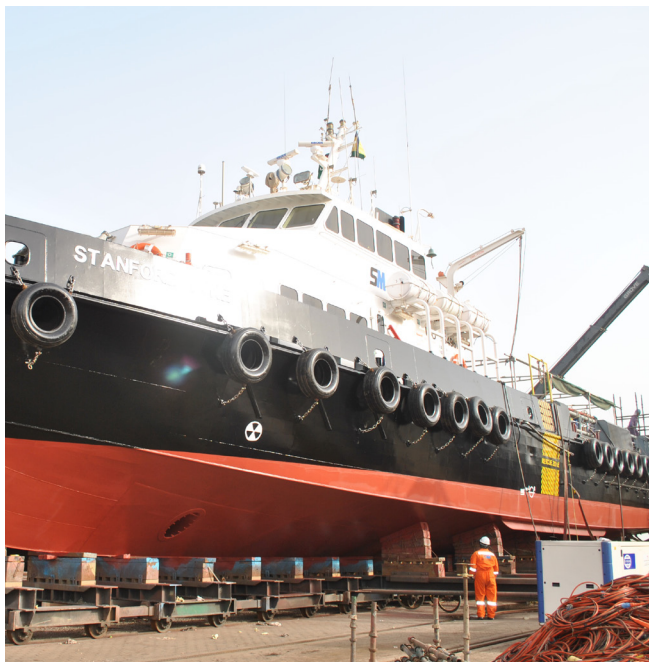
Stanford Rhine and Stanford Puma - 41M Fast Support Intervention Vessels under modification
